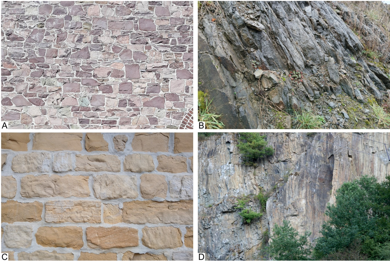
Figure 17. Illustration of some members of the Condroz Formation. A. Amaranth sandstone of the Citadelle de Huy Facies (Montfort Member) used as building stone. Strud, rue de Strud . B. Carbonate sandstone and siltstone of the Ciney Member. Leignon, section along the road N949. C. Yellowish weathered dolomitic sandstone of the Ciney Member, known as Pierre d'avoine in the Condroz, used as building stone. Sorée, Saint-Martin church. D. Thinly bedded micaceous sandstone typical of the Comblain-la-Tour Member, Comblain-la-Tour quarry.
