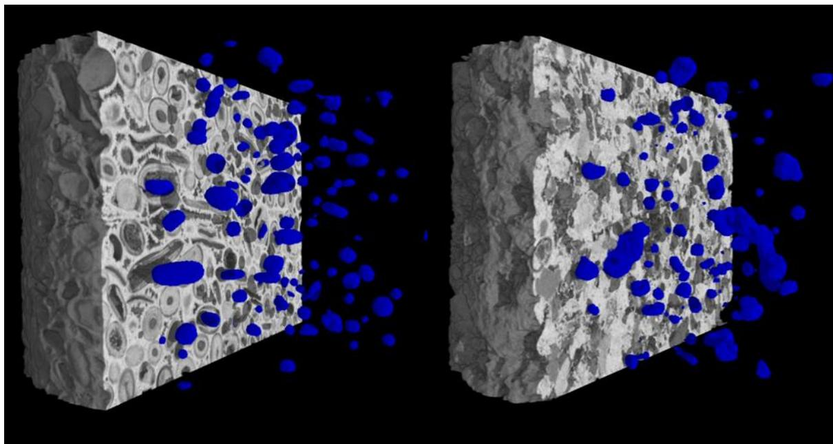
**Figure 1.** Vertical cross section of 3D  $\mu$ CT image through (left) Savonnières and (right) Tabaire revealing the 3D rendered volume of biogenic gas after one week of bacterial growth. Diameter of the samples is 6 mm.
