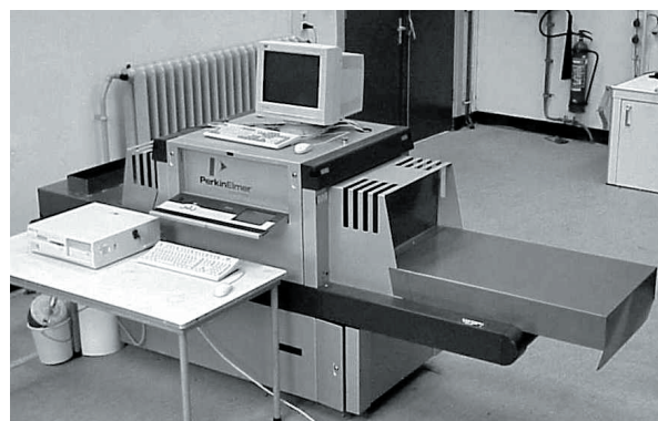
Figure 3. An airport security X-ray system that is converted for continuous inspection of bulk solids at the laboratory of Delft University of Technology. It combines dual energy XRT data with dedicated imaging algorithms for identification of a variety of materials. A typical belt speed for the system shown is approximately 0.5 m/s, belt width is 60 cm.
