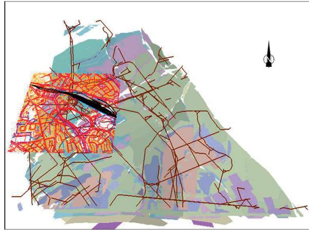
**Figure 8.** Tilted surface projection of panels and main stone drifts of the Oranje Nassau I colliery and the Heerlen city target area.
