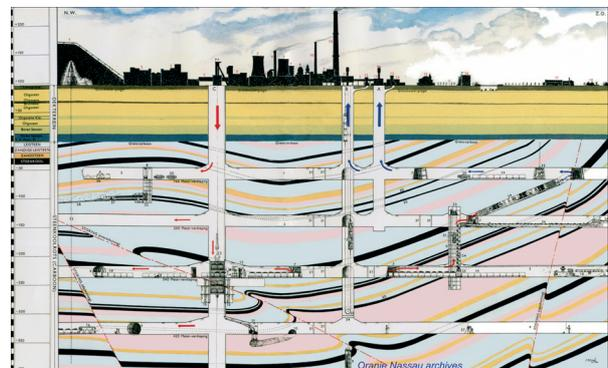
**Figure 2.** Schematic section of a coal mine. The main shafts, stone drifts, blind shafts and mined coal seams are integrated parts of the human induced, subsurface reservoir (yellow: overburden rocks; black: coal seams).
