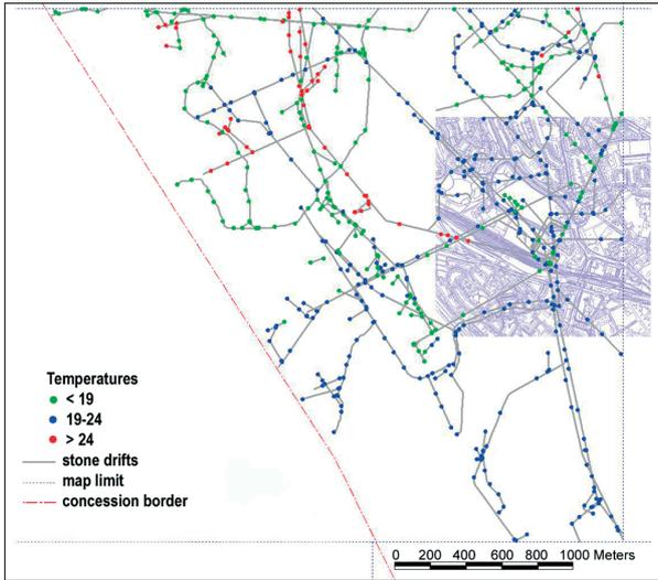
**Figure 7.** Calculated subsurface temperatures of the stone drifts in a part of the Oranje Nassau I colliery.
