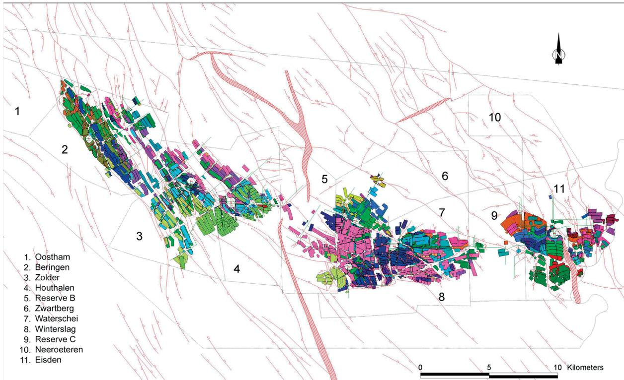
**Figure 5.** Belgian Campine basin: GIS surface projection of mined panels combined with mapped fault positions. Colours represent different mined coal seams.
