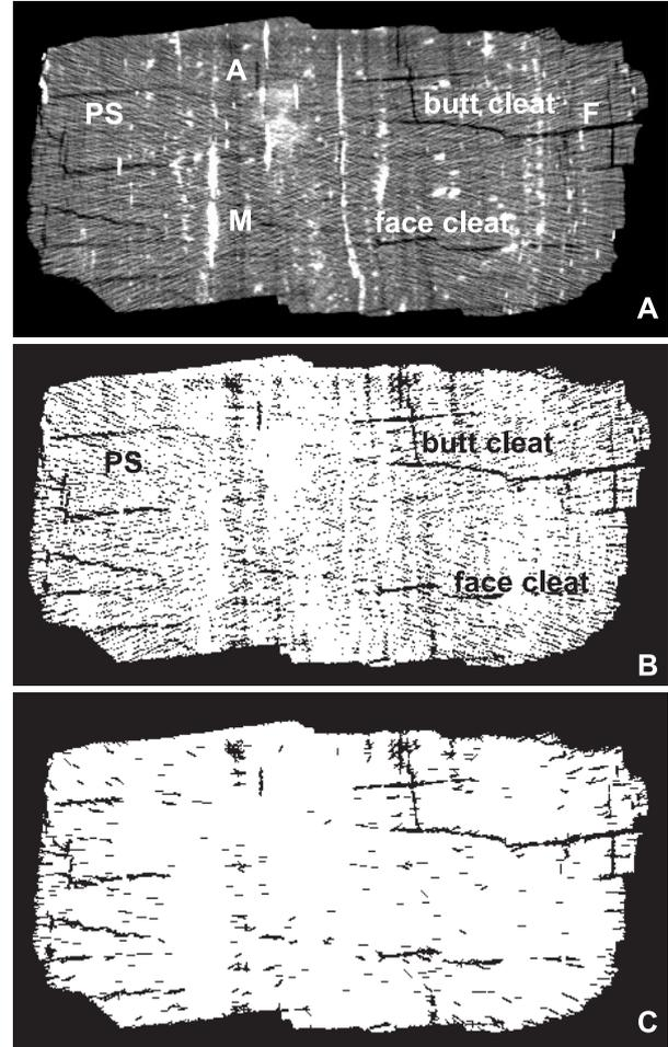
**Figure 7.** A: CT scan, showing black face- and butt cleats (F), white mineral filling (M), blurred cleats (A), distortion by photon starvation (PS). 7. B: Initial detection of the open cleats with artefacts. 7. C: Resulting open cleat system, after “linear open” procedure (no manual editing).
