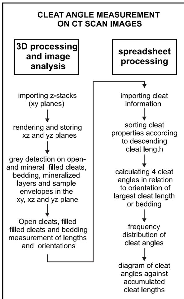
**Figure 6.** Flow chart of the image analysis procedure to define fracture angles from CT scans.
