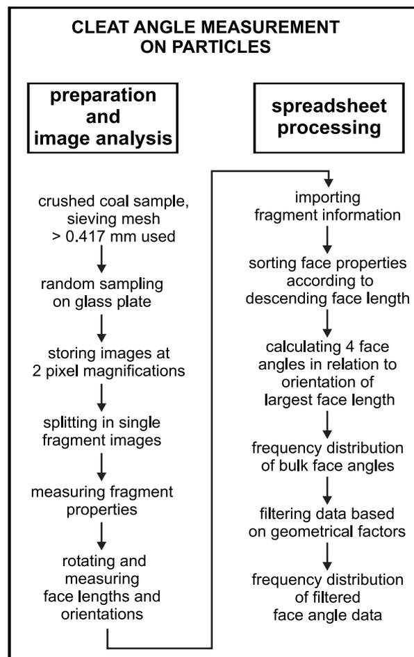
**Figure 1.** Flow chart of the image analysis procedure to define fracture angles from cuttings.
