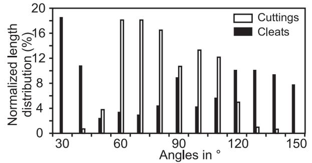
**Figure 10.** Angle distribution of sample 446 cuttings and the distribution of the open cleats of a limited amount (9) of CT-XY scans. This non-representative number of images results into an unpredictable response.
