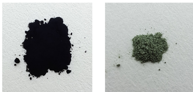
Figure 9: Pictures of the two as-synthesized powders: MoWOx 1h (left) and WO 3-δ 1h (right).
