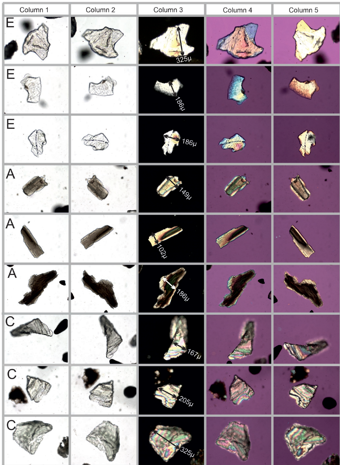
Figure 2: Photographs of the three most common volcanogenic mafic minerals of the Rocourt Tephra. Rows: E = enstatite; A = amphibole; C = clinopyroxene. Columns: (1) and (2) orthogonal positions in plane-polarized light to highlight pleochroism; (3), (4), (5) maximum illumination between cross-polarized light to highlight birefringence with intercalated gypsum (4) and (5).
