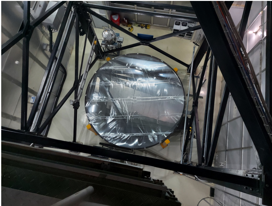
Figure 3: Top view of the ILMT, showing the liquid mercury mirror covered by a mylar film.
