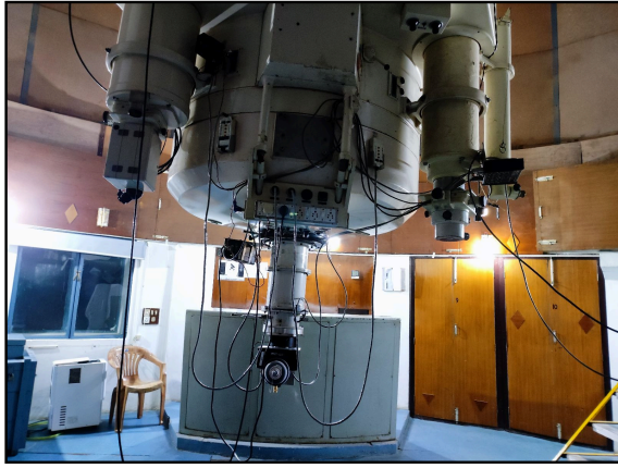
Figure 2: AIMPOL instrument mounted on 1.04 m Sampurnanand telescope in the left panel and the right panel represents the schematic optical layout of the instrument.
